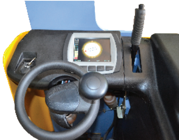
Electronic Power steering Battery indicator display & parking brake
